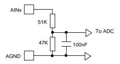
Figure 5 - Analog Input Circuit
